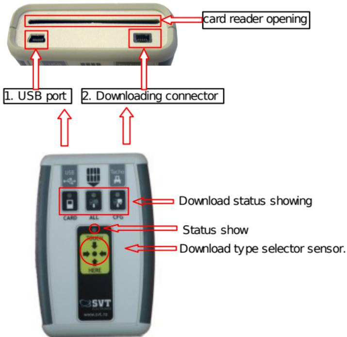
With the use of the touch sensor you can select the download type. You can use it only when downloading data from the tachograph.
