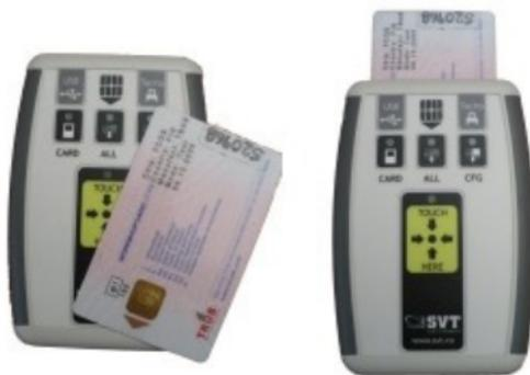
After about 5 seconds the **CARD** display will light up, and the statusle will start blinking in green.
